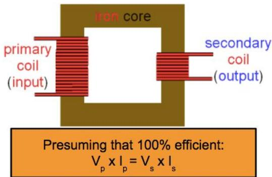
$$V_p = \frac{V_s \times I_s}{I_p} \quad I_p = \frac{V_s \times I_s}{V_p}$$
