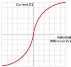
The graph for a filament lamp is not a straight line and therefore does not obey Ohm's Law. As more current flows in a lamp the metal filament gets hotter. The metal atoms in the filament vibrate faster and further from their positions. This results in an increase in collision with the travelling electrons hindering their flow and causing more resistance. This is shown by the flattening out of the graph as the current increases indicating that the resistance is increasing.
