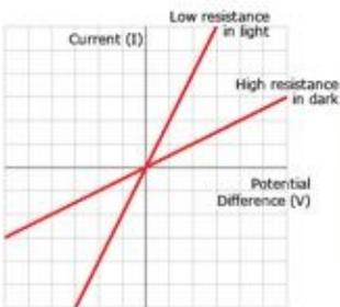
An LDR is a semi-conductor. When light shines on it releases electrons which increases the number of electrons to carry the current. Thus, as the light increases the current increases resulting in a reduction in resistance. In the dark however no extra electrons are available so the current experiences a greater resistance.
