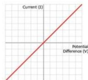
The graph shows the resistor is obeying Ohm's Law. The straight line tells us the current is proportional to the potential difference across the resistor.
